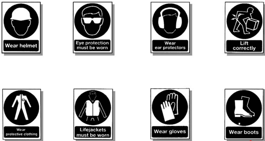
Fig. 1.10 Safety signs showing type of PPE to be worn.
