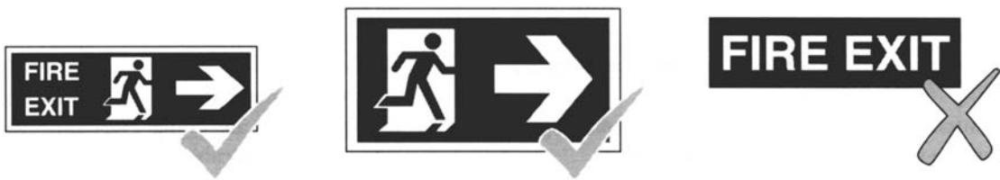
Fig. 1.12 Text only safety signs do not comply.
