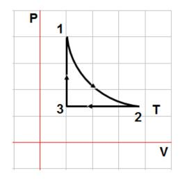
35. A sample of an ideal gas taken through a closed cycle is presented by the P-V diagram. The process 1-2 is perfectly isothermal. Which of the following is true about the change in internal energy and work done by the gas during the process 1-2?
