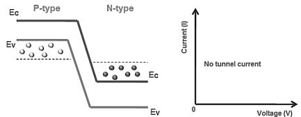
Figure: Unbiased Tunnel Diode
