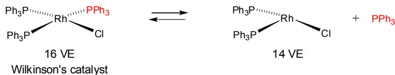
It loses a ligand, forming the T-shaped 14-valence electron Rh(+1) centre, prior to the oxidative addition of H<sub>2</sub>. It has to lose the PPh<sub>3</sub> ligand as it is quite bulky, and prevents the ready addition of H<sub>2</sub> to form a 6-coordinate RhCl(PPh<sub>3</sub>)<sub>3</sub>(H)<sub>2</sub>. This is **ligand dissociation**.
