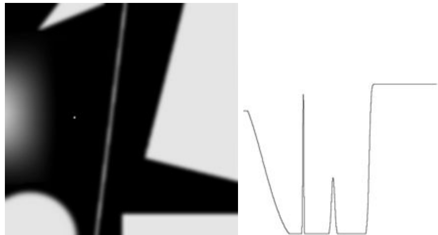
FIGURE 3.38 (a) A simple image. (b) 1-D horizontal gray-level profile along the center of the image and including the isolated noise point. (c) Simplified profile (the points are joined by dashed lines to simplify interpretation).
