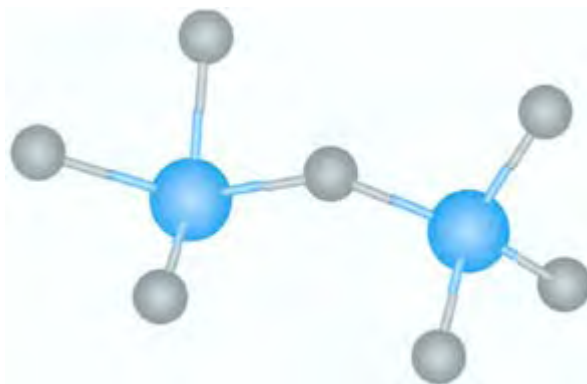
FIGURE 7.1 The zeolite building units. Two \text{SiO}_4/\text{AlO}_4 tetrahedra linked by corner sharing.
