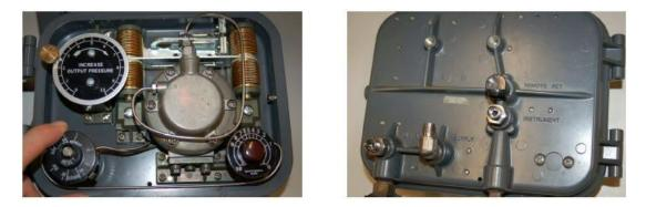
The mechanism is remarkably similar to the one used throughout the explanatory discussion, with the important distinction of being motion-balance instead of force balance. Proportional and integral control modes are implemented through the actions of four brass belows pushing as opposing pairs at either end of a beam:
