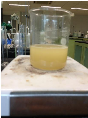
Figure 34: Soap solution with \text{NaNO}_3 being heated and stirred for 20 minutes
