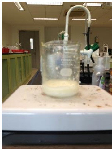
Figure 28: Soap solution with \text{NaNO}_3 being heated and stirred for 10minutes
