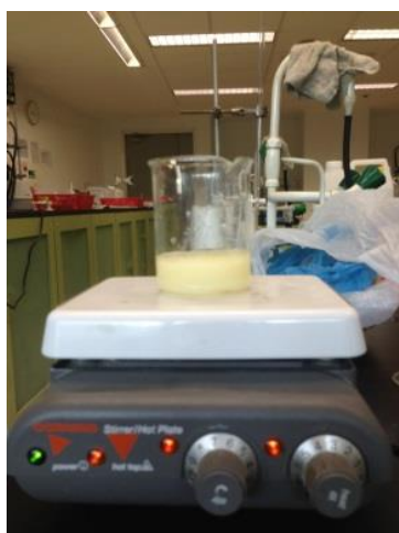
Figure 30: Detergent solution with \text{NaNO}_3 being heated and stirred for 10minutes
