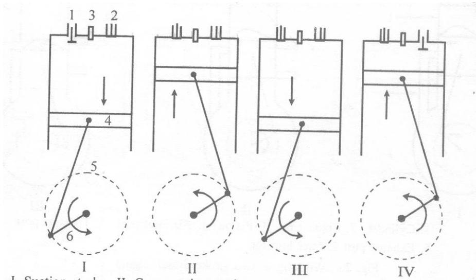
I Suction stroke II Compression stroke III Working stroke IV Exhaust stroke
