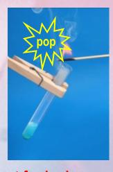
(test for hydrogen gas)
