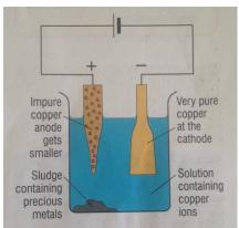
Figure 3 Many of these cells operate at the same time in industry. The cathodes are removed about every two weeks.
