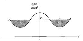
FIGURE 9.21 Water-filling interpretation of information-capacity theorem for a colored noisy channel.
