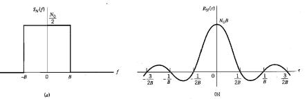
**FIGURE 1.17** Characteristics of low-pass filtered white noise. (a) Power spectral density. (b) Autocorrelation function.
