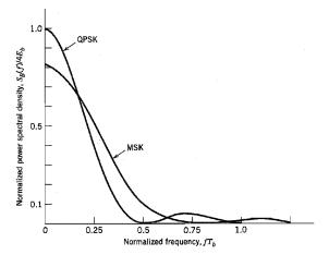
FIGURE 6.9 Power spectra of QPSK and MSK signals.
