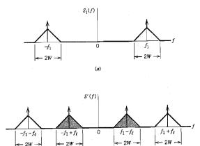
(b) **FIGURE 2.17** (a) Spectrum of modulated signal  $s_1(t)$  at the mixer input. (b) Spectrum of the corresponding signal s'(t) at the output of the product modulator in the mixer.
