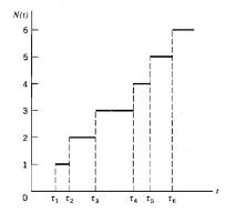
FIGURE 1.14 Sample function of a Poisson counting process.
