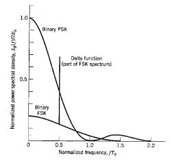
FIGURE 6.5 Power spectra of binary PSK and FSK signals.
