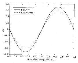
FIGURE 6.72 S-curve of NDA-ELD synchronizer measured under noiseless and noisy conditions.
