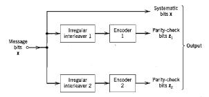
FIGURE 10.32 Block diagram of irregular turbo encoder.
