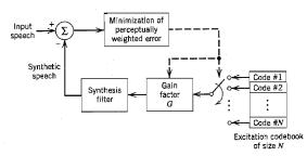
FIGURE 8.28 Encoder of the code-excited linear predictive codec (CELP): the transmitted signal consists of the address of the code selected from the codebook, quantized G, and quantized filter parameters.
