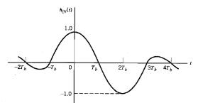
FIGURE 4.18 Impulse response of the modified duobinary conversion filter.
