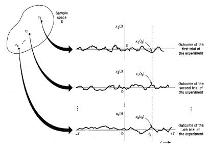
FIGURE 1.1 An ensemble of sample functions.
