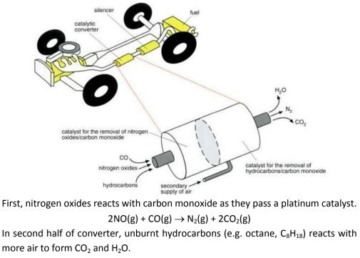
$2C_8H_{18}(g)+25O_2(g)\to 16CO_2(g)+18H_2O(g)$  CO<sub>2</sub>, H<sub>2</sub>O and N<sub>2</sub> are all non-pollutants. These reactions are all redox.
