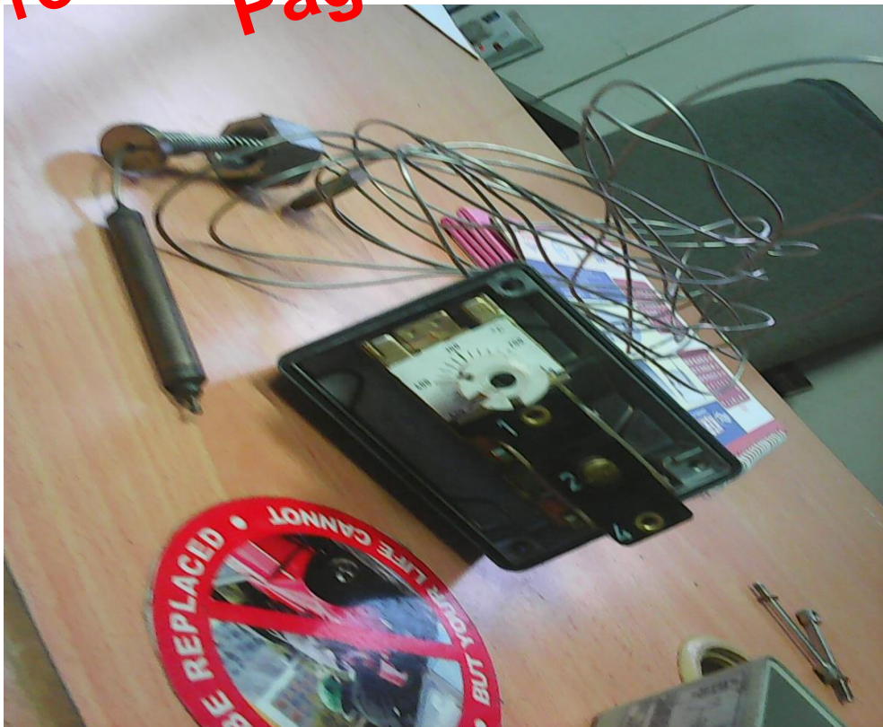
Figure 2-15b : Temperature switch showing probe
