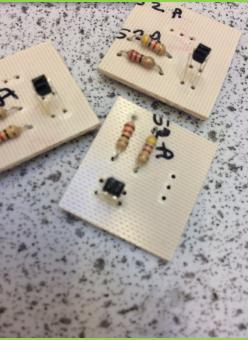
Once I had soldered all of the resistors I added the opto-isolators and soldered them into place.
