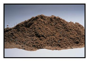
(a) Unit Weight (Bulk Density) and Voids -The weight of the organizate required to fill a container of a specified unit volume.
