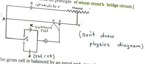
The emf of the given cell is balanced by an equal and opposite external potential so
