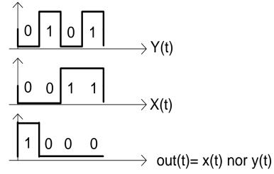
• Output value is the complemented output from an "OR" function.
