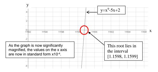
The interval has now been narrowed down to the acceptable level of accuracy (3 d.p.) – so the root is 1.160 to 3 d.p. as all values in the interval [1.1598, 1.1599].
