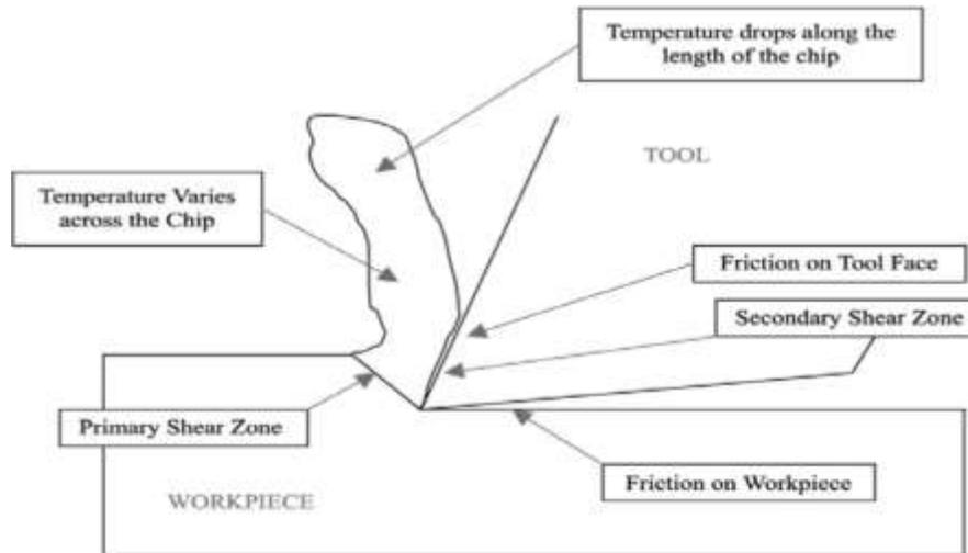
Fig: Schematic of chip formation
