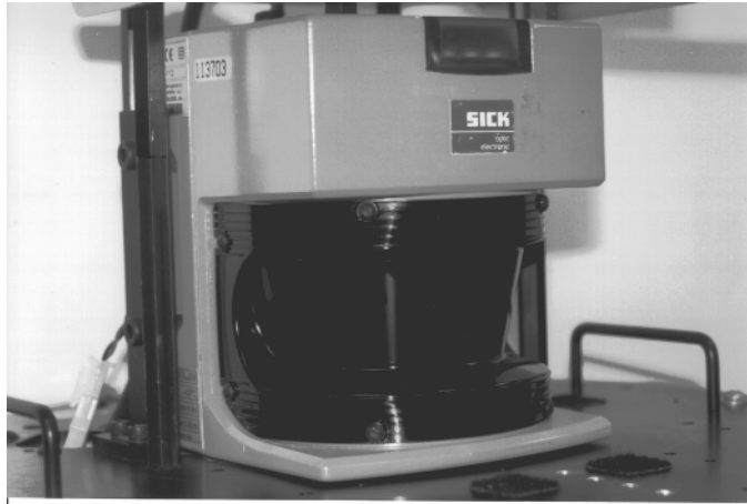
Figure 6.28 Sick laser, covering a 180^\circ area
