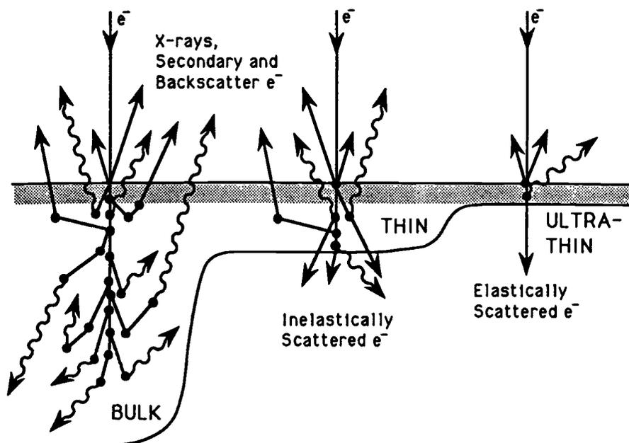
FIG. 1—Signal types generated by electron beams impinging on a sample of varying thickness. Adapted from Thomas [1].
