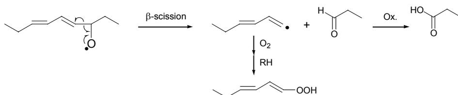
**Scheme 1.7:** Example of a  $\beta$ -scission reaction leading to chain breaking and formation of aldehydes and carboxylic acids.<sup>[57]</sup>
