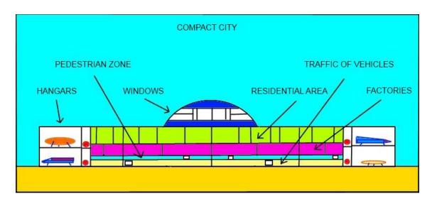
In this type of city transport vehicles would use the lower section. Located above section would be used for pedestrian traffic, to avoid the risk of abuse. On top of this section would be the area of factory and office work. Finally above all could be located residential areas where housing would be found.
