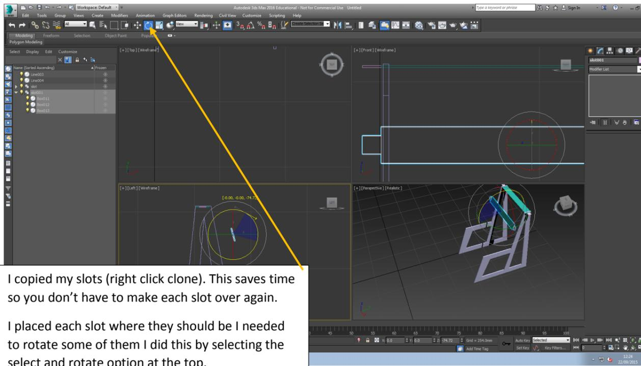
I copied my slots (right click clone). This saves time so you don't have to make each slot over again. I placed each slot where they should be I needed to rotate some of them I did this by selecting the select and rotate option at the top.
