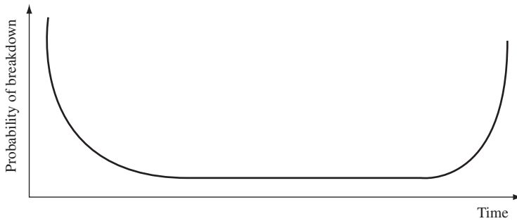
Figure 53.1 'Bathtub curve' showing the probability of breakdown with age
