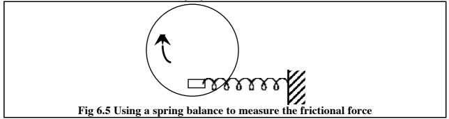
This apparatus made evident the fluctuations which occur in the friction force and showed that whereas at low velocities the friction force was essentially independent of the velocity, it did decrease when the velocity became high.
