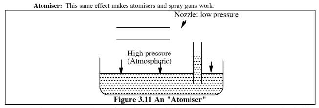
It is most important that the free surface of the liquid should be open to the atmosphere, else the high pressure outside the container and the low pressure inside will result in the container being crushed. {Fly sprays always have a small air hole.]
