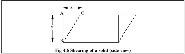
A solid deforms instantaneously and then stops deforming. When the shearing stress is removed, if the solid is elastic the deformation recovers.
