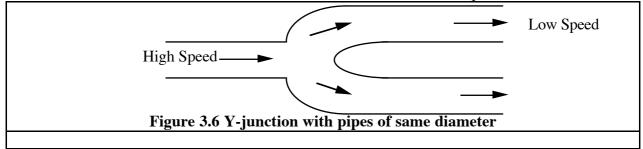
Conversely, if it is important to keep the flow speed up, the pipes after the branch must have half the cross-sectional area of those before.
