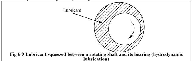
In this type of lubrication, the frictional energy loss is due only to the viscous forces in the lubricant (see post-lecture material). The viscosity cannot be reduced indefinitely, however, since the separation between the surfaces decreases as the viscosity decreases and eventually the surfaces come into contact.
