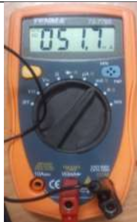
Figure 13: Full load - 51.7mA
