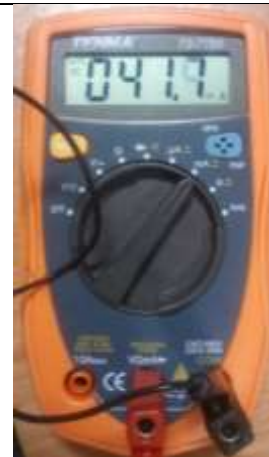
Figure 14: Part load - 41.7mA
