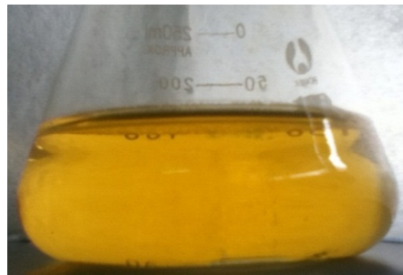
Figure 2: The colour of the solution after the CO 2 exhalation into the flask (yellow):
