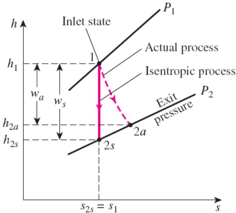
$$\eta_T = \frac{\text{Actual turbine work}}{\text{Isentropic turbine work}} = \frac{w_a}{w_s}$$
