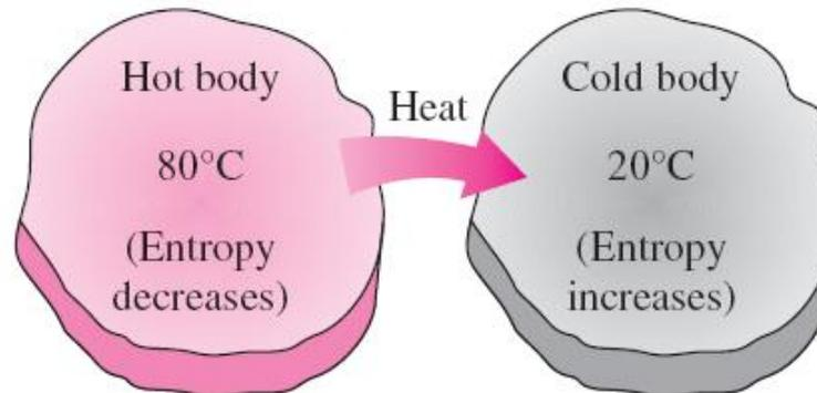
During a heat transfer process, the net entropy increases. (The increase in the entropy of the cold body more than offsets the decrease in the entropy of the hot body.)
