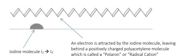
• A gap has been created within the polymer backbone which allows the lonely electron, now dissociated from the double bond, to move. This results in the double bond successively booing along the polymer backbone and a charge begins to flow. The positive charge is is to get electrostatic attraction to the iodide ion and is unable to move so readily.
