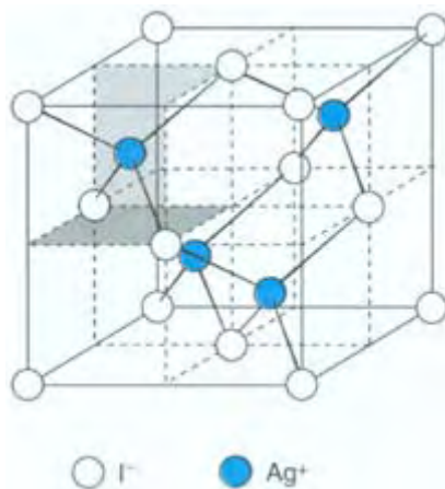
FIGURE 5.43 The zinc blende structure of \gamma -AgI.
