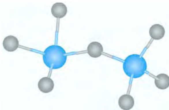
FIGURE 7.1 The zeolite building units. Two \text{SiO}_4/\text{AlO}_4 tetrahedra linked by corner sharing.
