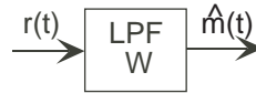
Figure 6.5: The receiver for baseband communication systems is quite simple: a lowpass filter having the same bandwidth as the signal.
