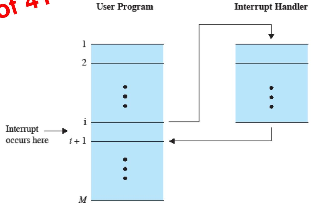
Figure 1.6 Transfer of Control via Interrupts
